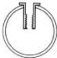
After drilling hole, tubular rivet is inserted.
