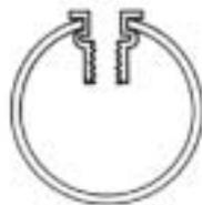
A header tool is then used to crimp the rivet inside the pipe wall.
